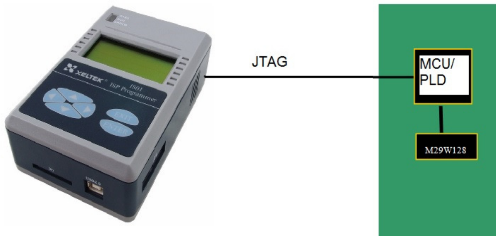
Programming Parallel NOR/NAND chip indirectly via JTAG: Non-Intrusive Method
